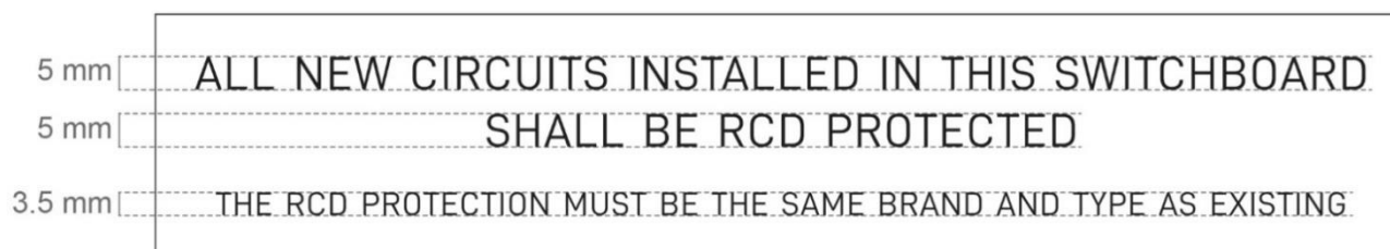
Figure 2. Label to display on all new Department of Education's distribution switchboards (not to scale)
